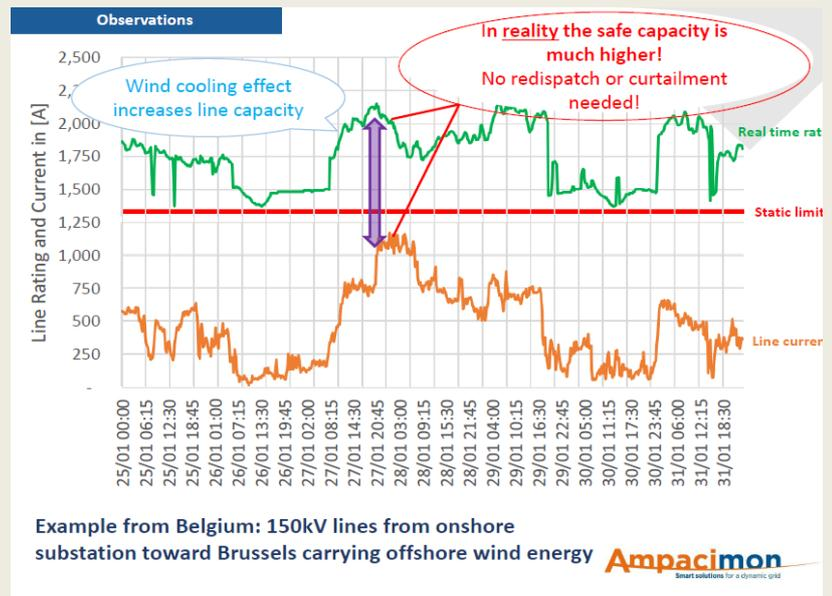
Figure 2. Differences between real-time DLR and Static Line Rating on Belgian Transmission Line. (Rena Kuwahata. Ampacimon 2020)
